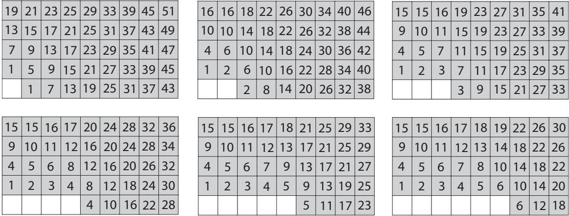
Figure 7: Results from the dynamic program for six configurations. Entries in each cell indicate the number of escort-moves required to bring the item to the I/O point, which is the bottom left cell.
